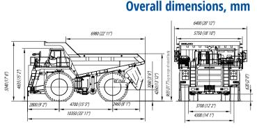
Overall dimensions are specified for basic configuration of the dump truck.
